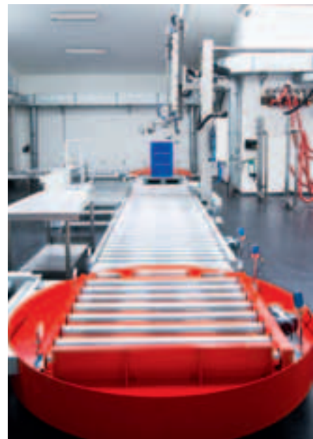
In the clean room, the air pressure is kept on a constant level and, through the use of various air locks and ventilation systems, free of germs.
